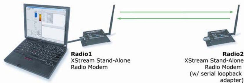
Figure 30: Hardware set-up for RF communication test between Radio1 (located at weather station site) and Radio2 (located at LAS-Receiver site).
