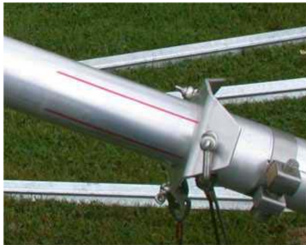
Figure 6: Clamping zone of mast sections are indicated by red stripes printed on the mast sections.
