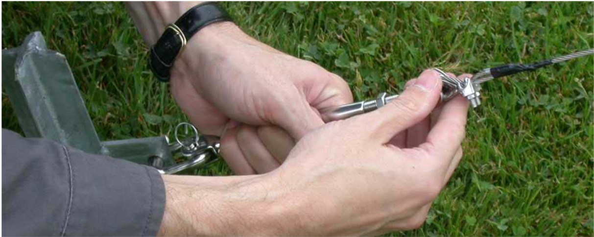
Figure 10: Fine adjustment of the spanner for levelling the mast.
