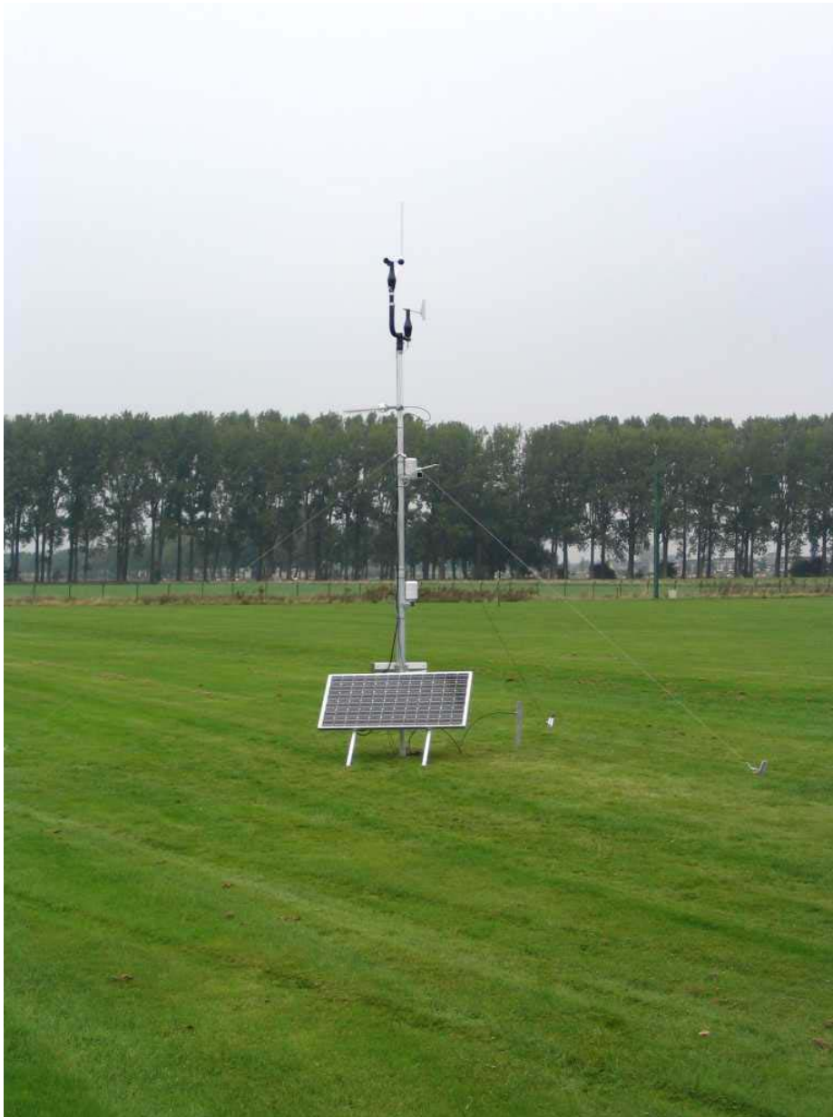
Figure 17: Operational weather station of LAS-RET system.
