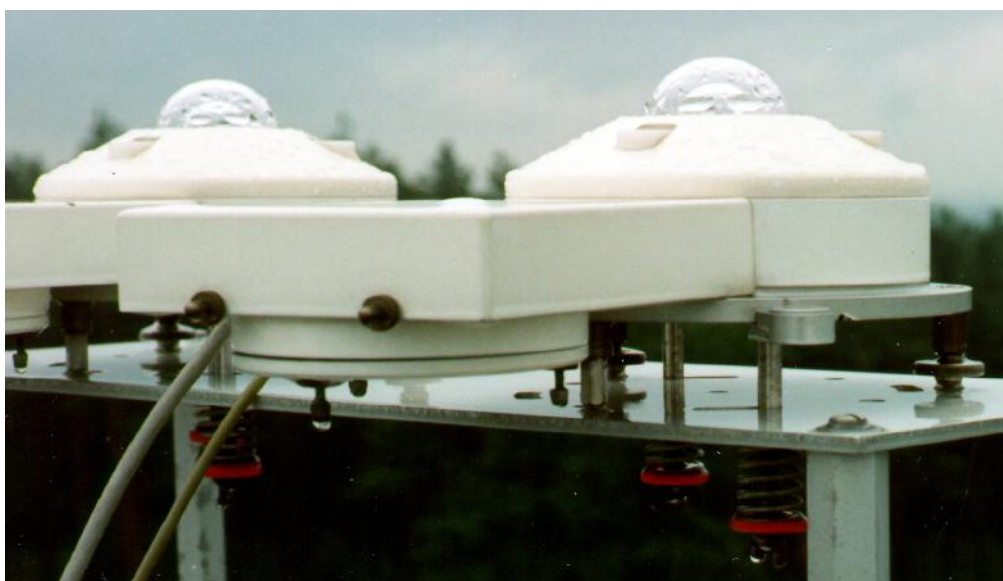
Figure 4.1. Ventilator with motor located beside the instrument as used by Deutscher Wetterdienst.
