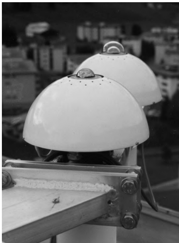
Figure 4.2. Ventilator with the motor located beneath the instrument. Note the extra ventilation holes near the top of the housing used to reduce snow accumulation (Davos, Switzerland).
