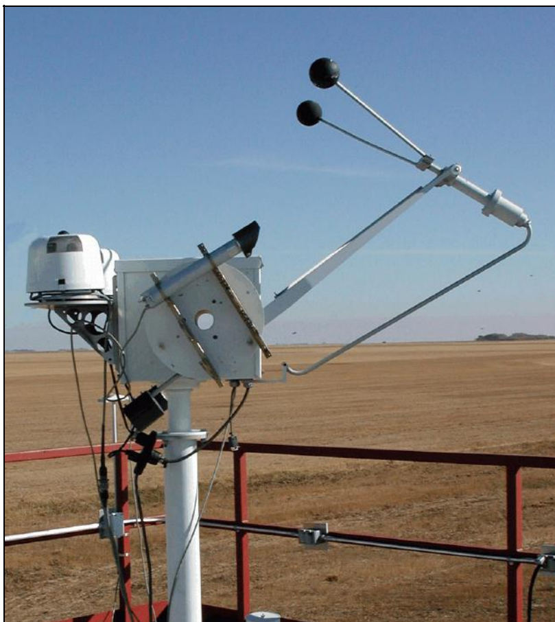
Figure 4.6. Canadian computer-controlled, friction-drive tracker used for measuring direct beam, diffuse and infrared radiation using a shaded pyrheliometer. The pyrheliometer mounting block is capable of holding three instruments, including an active cavity radiometer. A second mounting place is mounted on the opposite side of the tracker.
