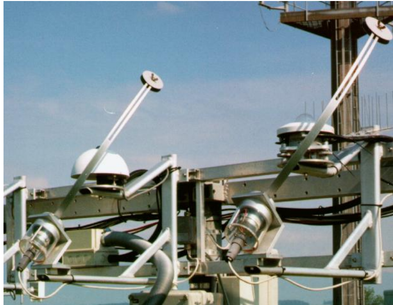
Figure 4.4. View of two Swiss oversized tracking disks. Note how the pyranometer is physically separated from the motor and the shade device. The increased width of the arm holding the shade disk eliminates the need for stabilizing wires, but increases the amount of sky obscured. The slot along the arm is for the movement of the shade disk. On the instrument to the right of the photograph, the vertical wires are used to deter birds perching on the instrument. (Courtesy of MeteoSwiss, Payerne, Switzerland.)
