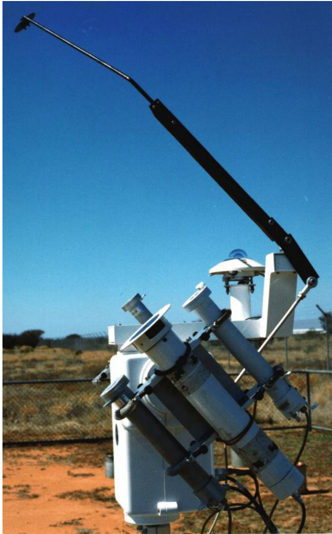
Figure 4.5. Australian active tracker used for both diffuse and direct beam measurements. This tracker is shading a single pyranometer, and pointing two normal incidence pyrheliometers and a GAW PFR sunphotometer on one side of the tracker and another pyrheliometer on the far side of the tracker. An active-eye is also situated on the far side of the tracker. (Courtesy Bureau of Meteorology, Australia)
