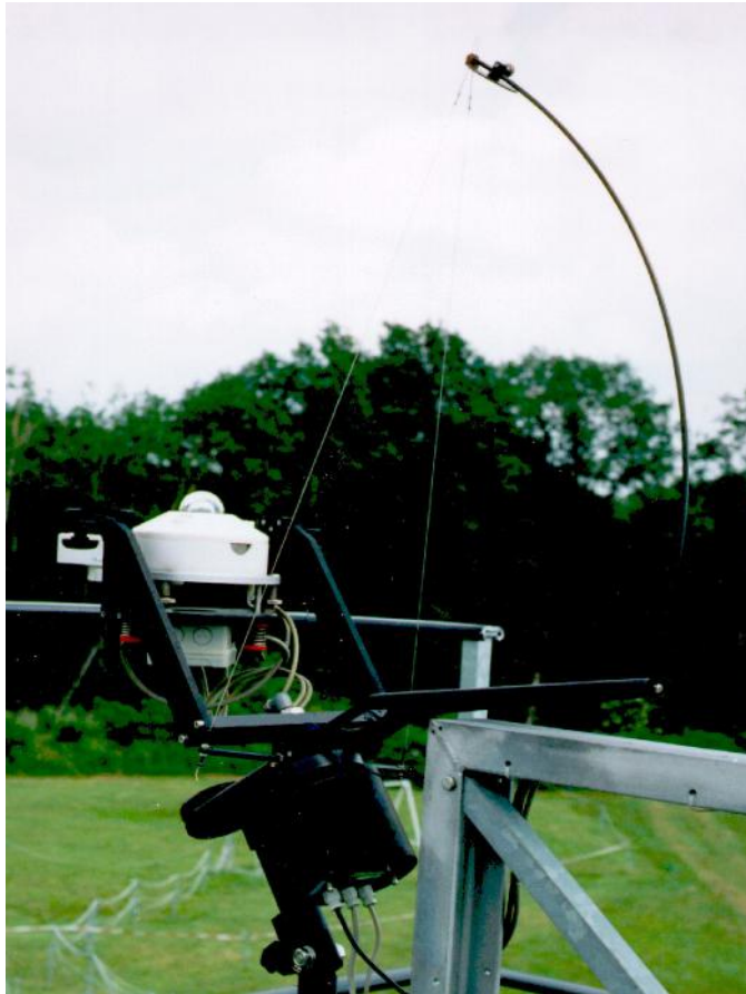
Figure 4.3. An one-axis tracker used in shading a pyranometer. Note the use of two fine wires to maintain the stability of the shading disk. (Developed by Deutscher Wetterdienst).
