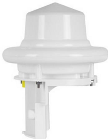
Radar reflection method to measure velocity on hydrometeors by 24-GHz-Doppler radar.
