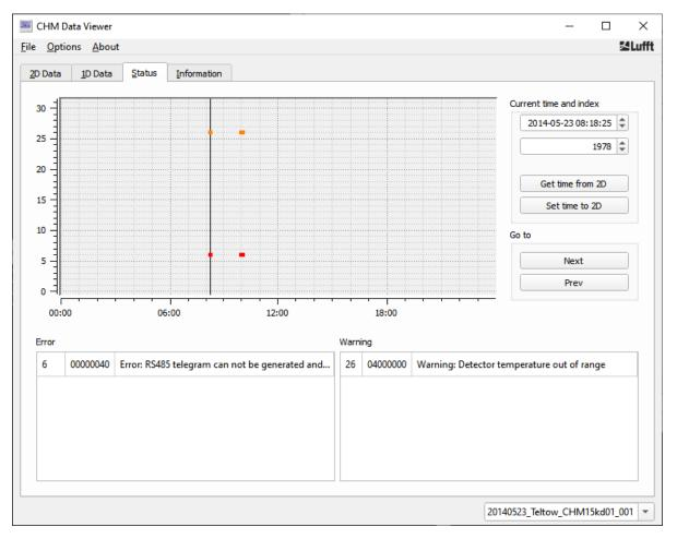
In the Status tab, the 31 bit status codes are visualized. In the time raster plot all bits set in the status code are shown as solid lines, error bits are red, warnings orange. The two tables in the lower part display the set error and warnings bits at the current time index, respectively. The current time index can be changed using the black link in the plot or the Current time and index input fields.
