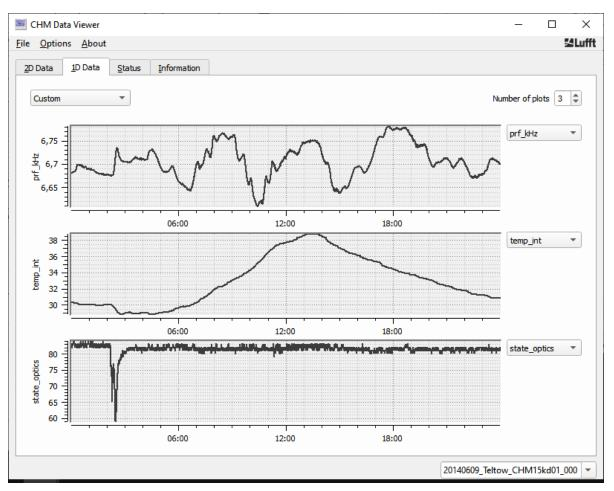
The 1D Data tab displays one-dimensional time-dependent variables from the NetCDF file. The combo box in the upper left corner selects one of the four following predefined scenarios:
