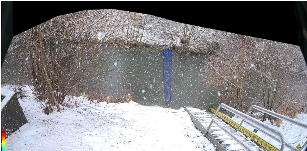
Image 13: HydroSight Flow - Velocity measurement at snowfall conditions
