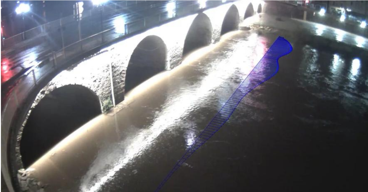
Image 11: HydroSight Flow - Nighttime measurement with surrounding whitelight
