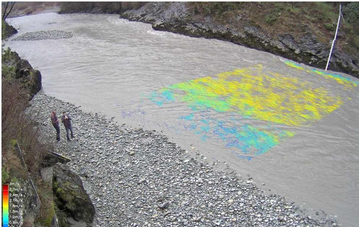
Image 8: HydroSight Flow - Velocity Vectors
