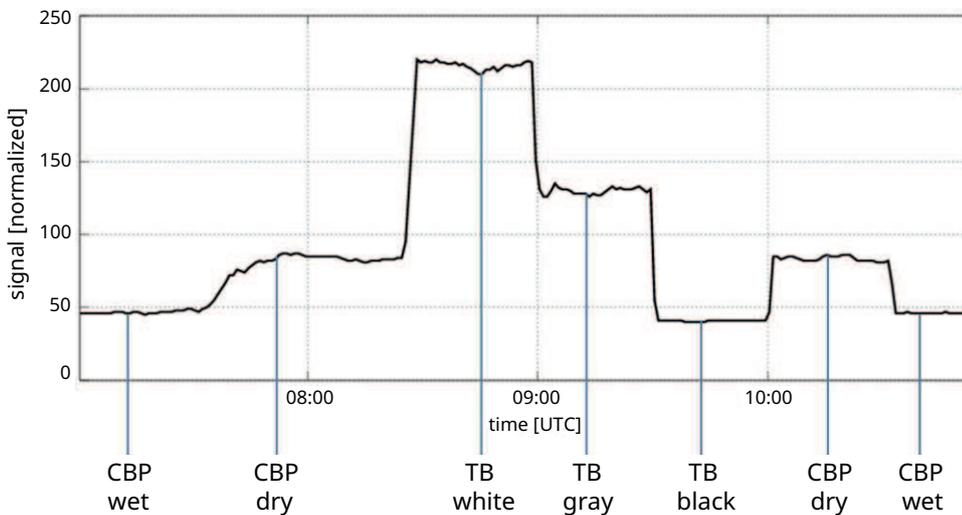
Variation of the signal intensity using different target plates. BP: Base plate, TP: Target plate
