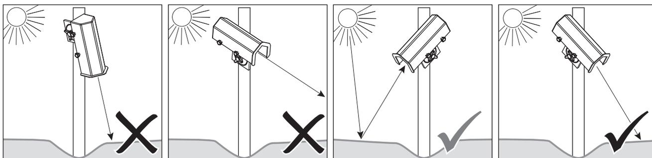
This prevents that snow falling from the mast or the device itself from affecting the measured result. If an angle is too large, this causes the laser beam to hit the ground at too flat an angle, which may give a vague and inconsistent distance measurement result. The larger the tilt angle, the more the snow depth calculation is influenced by the angle measurement.
