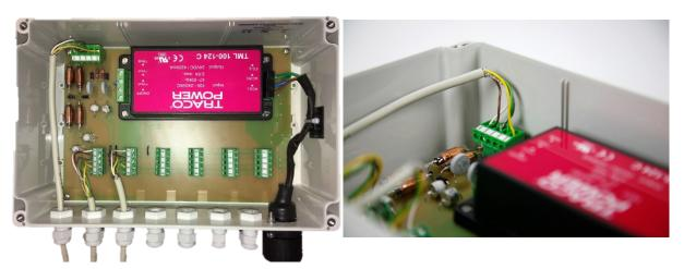
Do not forget to tighten the cable glands to ensure a waterproof installation.
