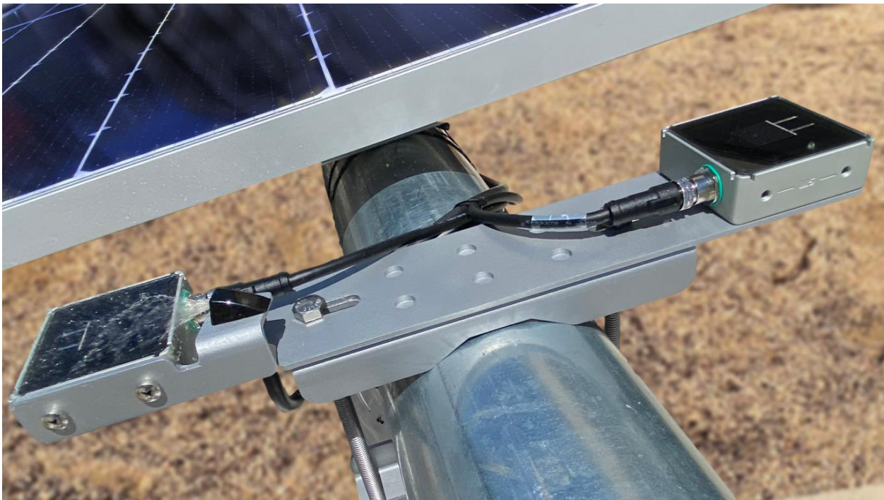
Figure 1-2: A washed and soiled reference cell pair for soiling measurement
