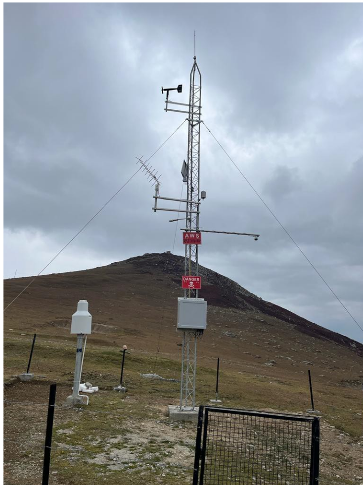
Figure 25. Example of a tower with a cautionary sign
