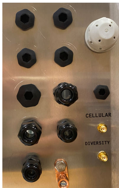
Figure 42. Example of glands on the enclosure
