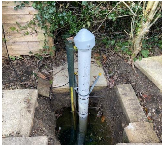
Borehole tube containing the ecoLog 1000 unit used by the Standlake residents to challenge the building development.
