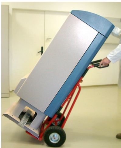
Figure 9 Transport with hand truck.
