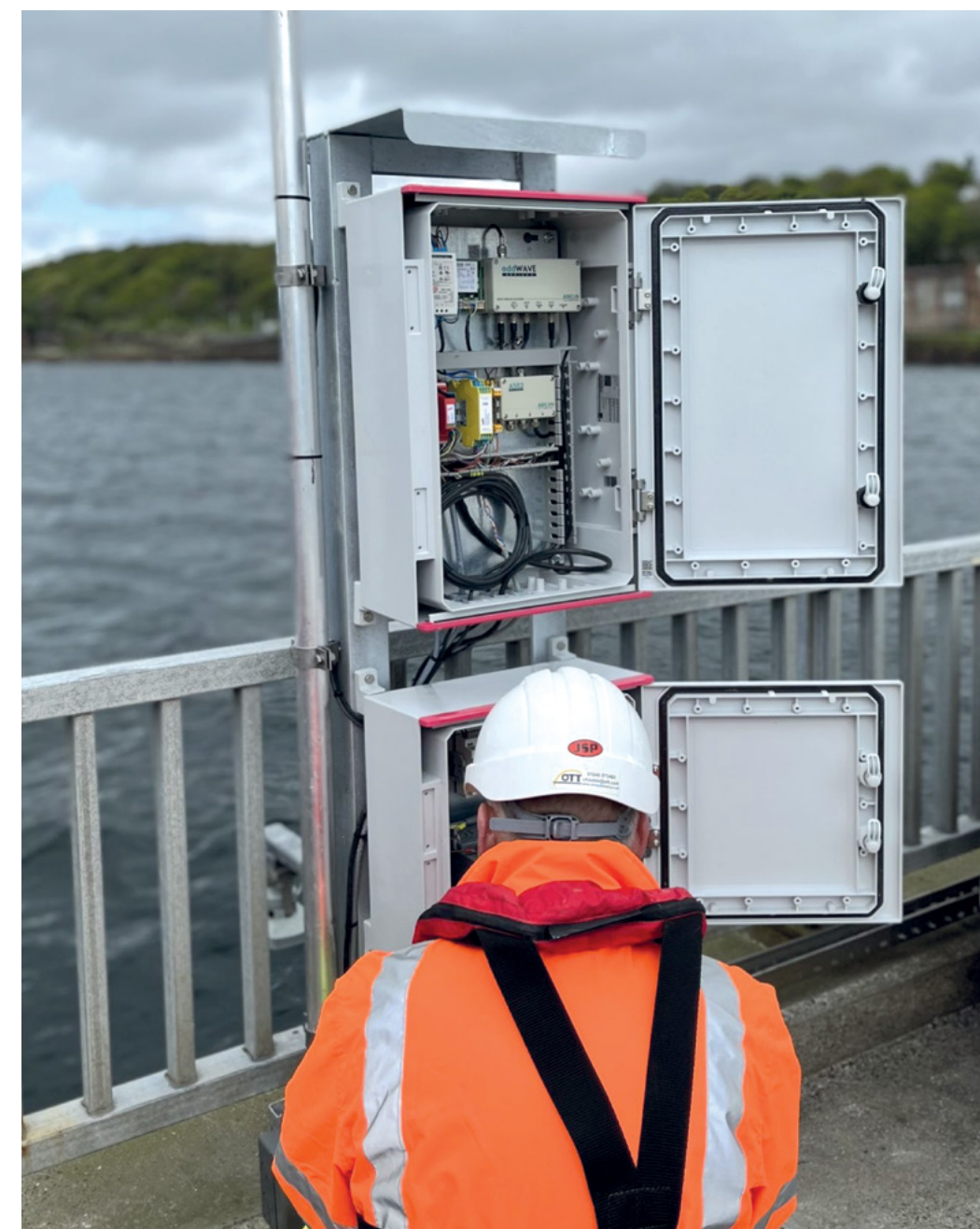
Hach and OTT HydroMet teams of service engineers can provide field maintenance and swap-in calibrated sondes.
